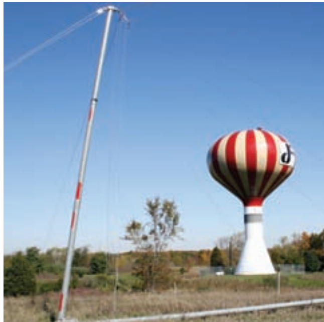
Developing alternative, renewable energy sources is an important field for the future. JCC is taking its first step toward exploring new alternative energy sources with the installation of an anemometer — a device for measuring wind velocity— on the south side of campus off Kimmel Road.
